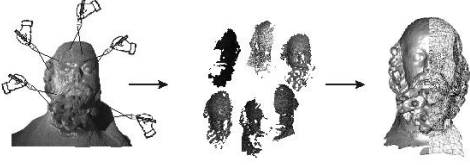
Figure 1: Range images from different viewpoints have to be transformed into the same coordinate system.
